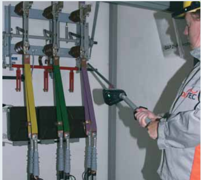
PHE Voltage Detector with visual indicator.
